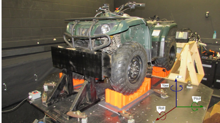
Figure 7: ATV seen in its safety restraints. The orange tire chocks are seen under the tires. The large tire wedges restrict the rotation of the rear tires. The global coordinate system is shown in the right corner.
